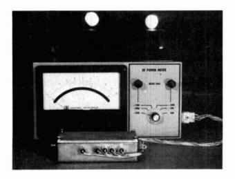
fig. 2. RF detector and amplifier mounted in a shielded enclosure. Range selection, meter and power supply are in a separate unit.
